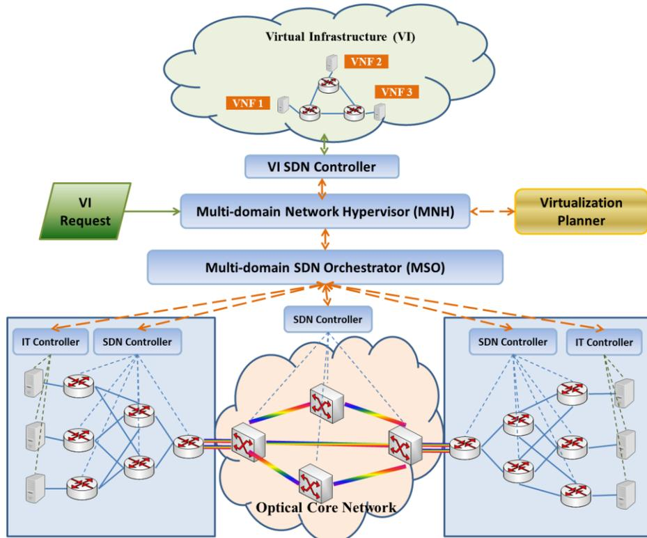
Figure 1: Virtualization and Orchestration Platform for SDN-enabled VIs and NFV services
