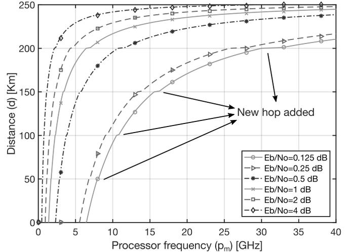
Figure 2: Maximum distance between an RRH and the BBU responsible for processing its signals, as a function of available processing capabilities available at the BBU and the SNR experienced on the wireless channel.
