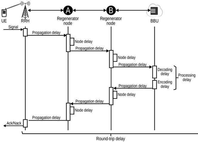
Figure 1: Round-trip delay components in a C-RAN.
