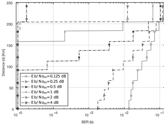
Figure 3: Maximum distance between an RRH and the BBU responsible for processing its signals, as a function of the target BER and the SNR experienced on the wireless channel.
