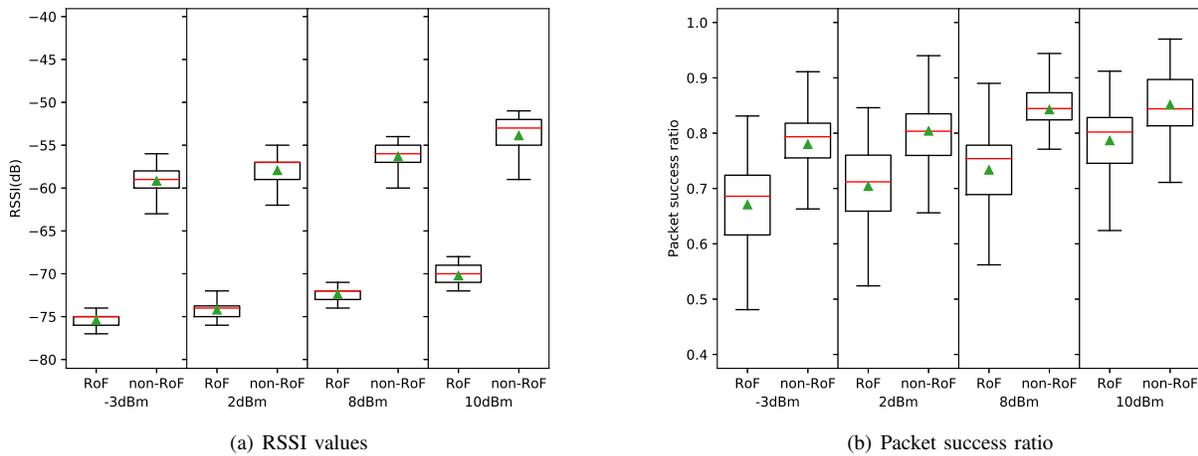
Figure 6. Impact of RoF system on the network performance. Distance between sensor node and antennas of 11 m in a NLOS scenario (wall on the middle).
