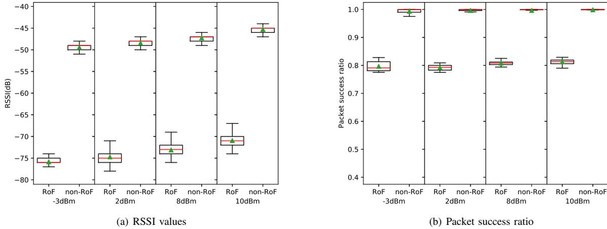
Figure 5. Impact of RoF system on the network performance. Distance  $d$  between sensor node and antennas of 8m in a semi-NLOS scenario.
