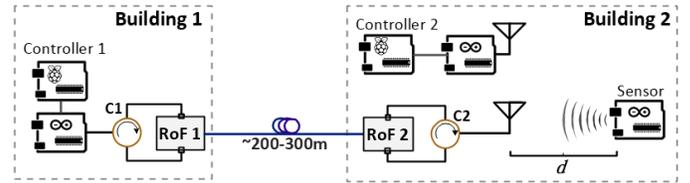
Figure 2. Experimental setup for the spatial-based methodology.
