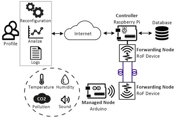
Figure 1. Overview of the FUTEBOL RoF-based IoT environmental monitoring testbed
