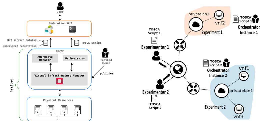
Fig. 1: O2CMF software stack and demonstration scenario for orchestrating NFV solutions.
