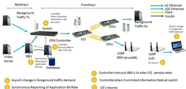
Fig. 2 Flexible-rate fronthaul system developed in the TCD testbed [4].
