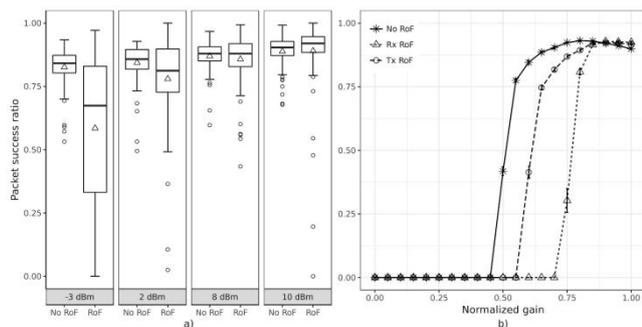
Fig. 9 Impact of RoF on IEEE 802.15.4-based technologies; a) XBBE-based results; b) USRP-based results.
