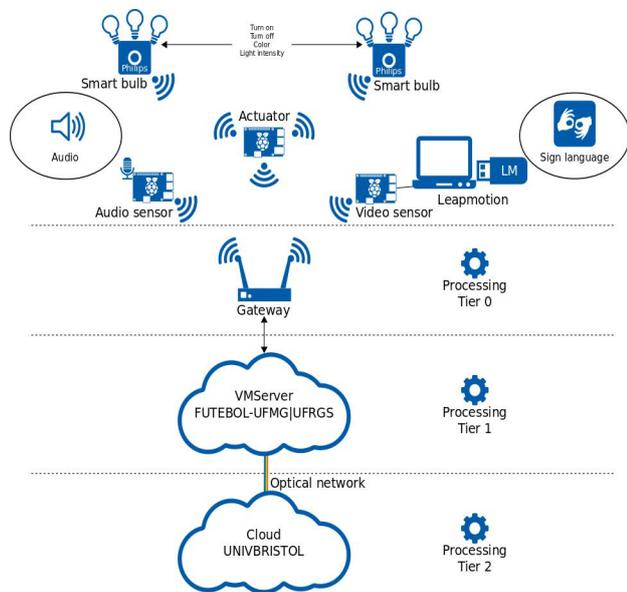
Fig. 7 Setup for adaptive Cloud/Fog experimentation.
