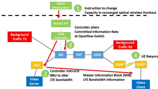
Fig. 1. Event diagram of the orchestrated control on the TCD variable-rate fronthaul testbed.
